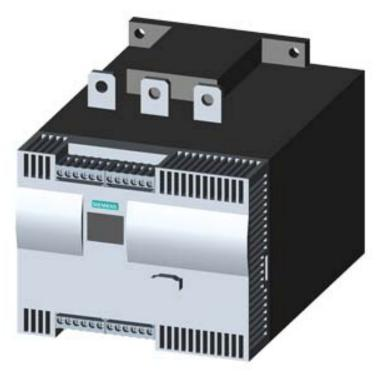
SIRIUS soft starter Values at 400 V, 40 °C Standard: 356 A, 200 kW Inside-delta: 617 A, 355 kW 200-460 V AC, 230 V AC Screw terminals
